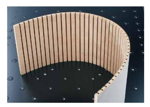
This option saves you an entire production step in subsequent processing. This is because your saw will also groove the panel material.
